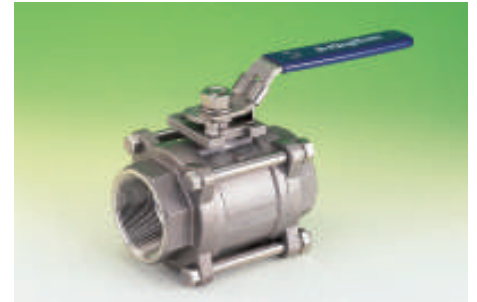
FIG. S-331T/C-331T: THREADED ENDS, 1000 PSI (69 BAR) W.O.G., ISO 5211 MOUNTING PAD.
