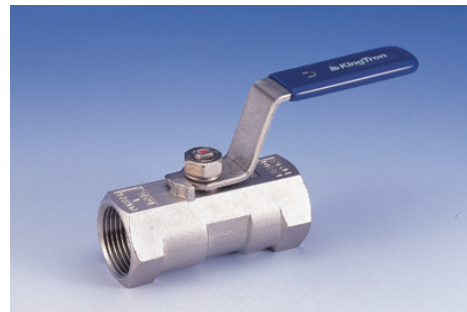
FIG. S-141T / C-141T: THREADED ENDS, LENGTHENED BODY, 1000 PSI (69 BAR) W.O.G..
