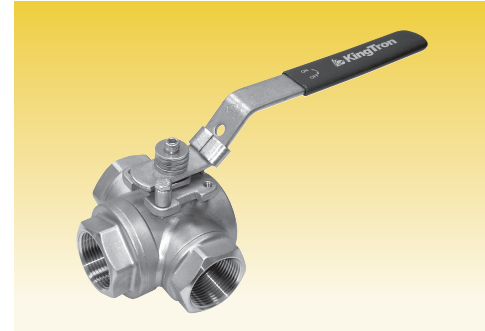
FIG. S-451T-T / C-451T-T: THREADED ENDS, T PORT, 1000 PSI(69 BAR) W.O.G., ISO 5211 MOUNTING PAD.
