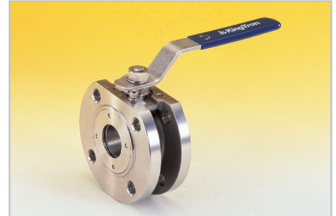
FIG. S-138W / C-138W: WAFER TYPE, PN16 FLANGED ENDS, ISO 5211 MOUNTING PAD.
