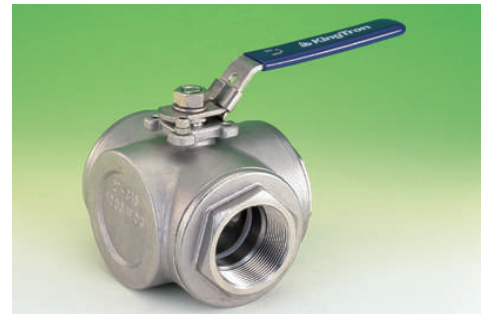
FIG. S-433T-T / C-433T-T: THREADED ENDS, T PORT, 1000 PSI(69 BAR) W.O.G., ISO 5211 MOUNTING PAD.
