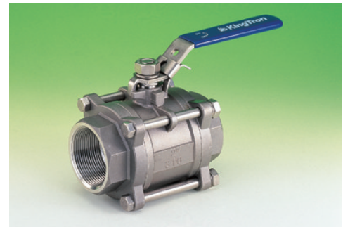
FIG. S-302T / C-302T: THREADED ENDS, 1/4" TO 2": 2000 PSI (138 BAR) W.O.G., 2 1/2" TO 3": 1500 PSI (103 BAR) W.O.G..
