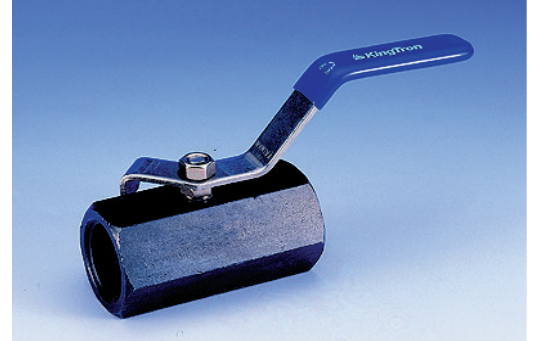
FIG. A-122T : THREADED ENDS, 2000 PSI (138 BAR) W.O.G., BARSTOCK BODY.
